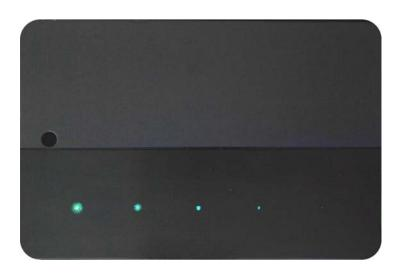
Test panel NR-5 is manufactured in accordance with the specification Pratt-Whitney Aircraft Drawing Number **TAM 146040**. Therefore test panel Nr-5 is comparable with test panel PSM-5.
