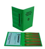
Laminated Magnetic Flux Strips are stiffer than QQIs, and do not conform to curved surfaces easily. But unlike QQIs, Laminated Magnetic Flux Strips are not permanently affixed to a part so they can be reused for multiple applications.
