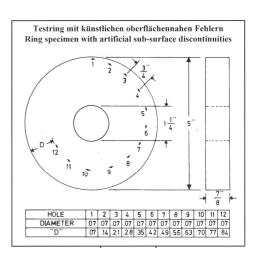
12 holes (diameter 0,07" (1,78mm) are placed on different distances from the outer cylindrical surface. When current (FWDC or HWDC) is passed through the central conductor, (conductor diameter 1 3/16 ", conductor length mustn't be less then 400mm), waste fields appear, decreasing as the distance from the hole to the outer cylindrical surface increases. When the magnetic suspension is applied on the disk, magnetic powder accumulates over the cylindrical surface holes, forming indicator lines.
