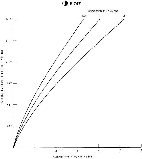
FIG. X1.2 Conversion Chart for 1-T Quality Level Holes to % Wire Sensitivity
