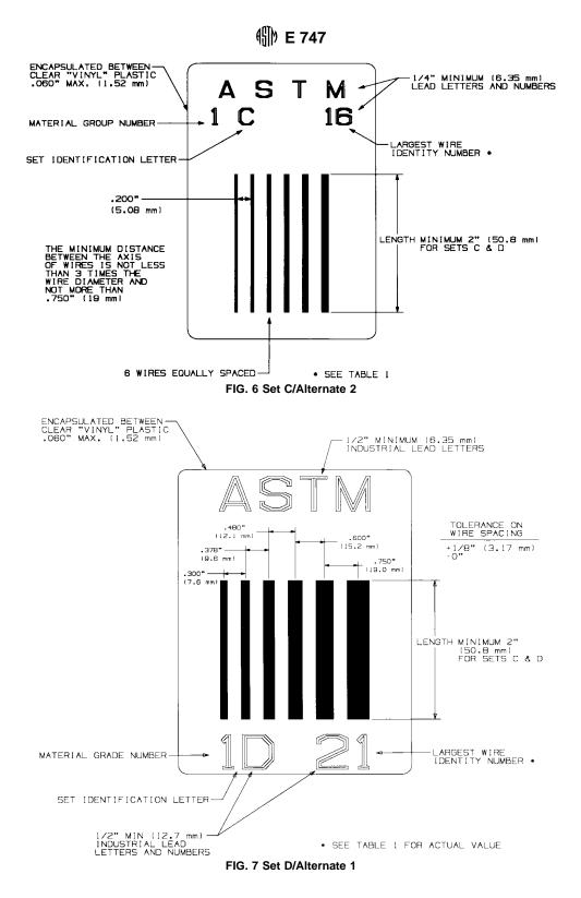
70 to 30 nickel-copper alloy (Monel)<sup>8</sup> (Class A or B of Specification B 164) or equivalent, or 70 to 30 copper-nickel alloy (Alloy G of Specification B 161) or equivalent.
