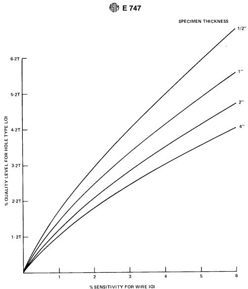
% SENSITIVITY FOR WIRE IQI FIG. X1.1 Conversion Chart for 2-T Quality Level Holes to % Wire Sensitivity
